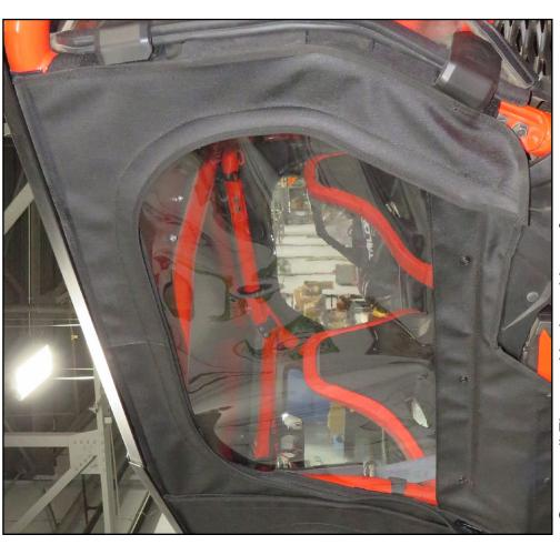
Secure all Flaps to Hook and Loop fastener.
