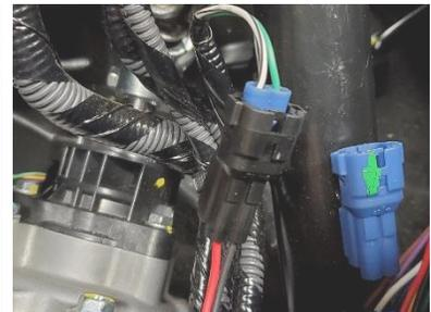
3. Install the Power Harness. Next to the Power Steering unit is a blue connector, un-plug the blue connector from the holder by lifting on the small center tab, plug the Power Harness in
