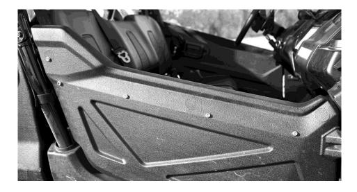
4. To use door simply unzip it and pull down on it to release the magnets then reach in and open the plastic door. Once in lift door up so the magnets attach to the bar and zip closed.
