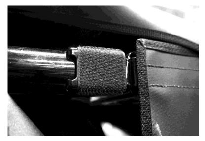
2. Then take the Rear Door and zip it to the Middle Rear Window. This ensures the door is properly placed. Then attach the top front corner to the Velcro. See photo below.
