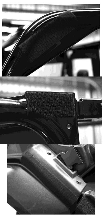
2. Next hold the door up to the frame and attach these spots then continue attaching it using the double-sided Velcro strips sewn perpendicular to the edge of the door. At each of the double-sided strips take one of the 3" adhesive Velcro strips and adhere it to the inside of the frame. Then wrap the double-sided strip around it so that the adhesive strip holds it firmly in place. The following diagrams show how it should look.
