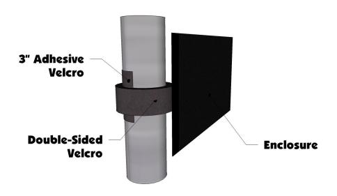
5. Begin installation of the Door Panels by hanging them from the Double-Sided Strips along the top of the doors. Hold the door up and mark where the each strip is and wrap a 3" adhesive strip around the roll cage. Now hang the door up and it will be in place to install the rest of the Velcro for the door. See Photo Below:
