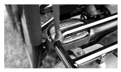
16. Next take the top and place it on the vehicle and run the straps through the buckles sewn to the corners. The photo below shows how this is done.
