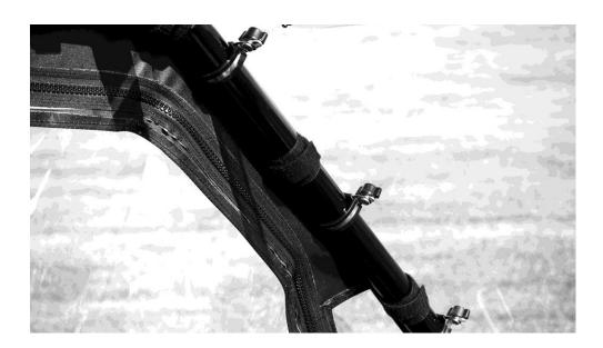
7. The rear of the door panel has 4 double-sided Velcro tabs that attach to the rear bar. For these you will take the two 6", 9", 10", and 15" adhesive Velcro strips and attach them down the rear bars facing the rear of the vehicle. Then attach the tabs to the bar as shown in the photo below.
