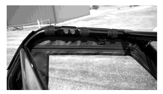
6. Now move around the door and attach the remaining Velcro strips in the same manner. Down the front of the door place the edge of the door against the side of the windshield and run the Velcro strips under it with the 3" adhesive Velcro on the inside of the roll cage.
