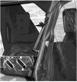
15. The rear straps will attach to the rear rack of the Pioneer. Put the looped end of the strap around the bar and run the other end of the strap through the loop. The photo below shows how this should look.
