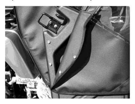
10. Next do the same for the three snaps along the bottom rear corner of the door as shown in the photo below.
